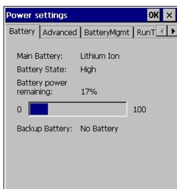
Figure 31: Power Settings — Battery Tab
