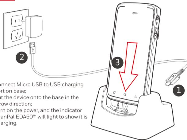
1. Connect Micro USB to USB charging port on base;
